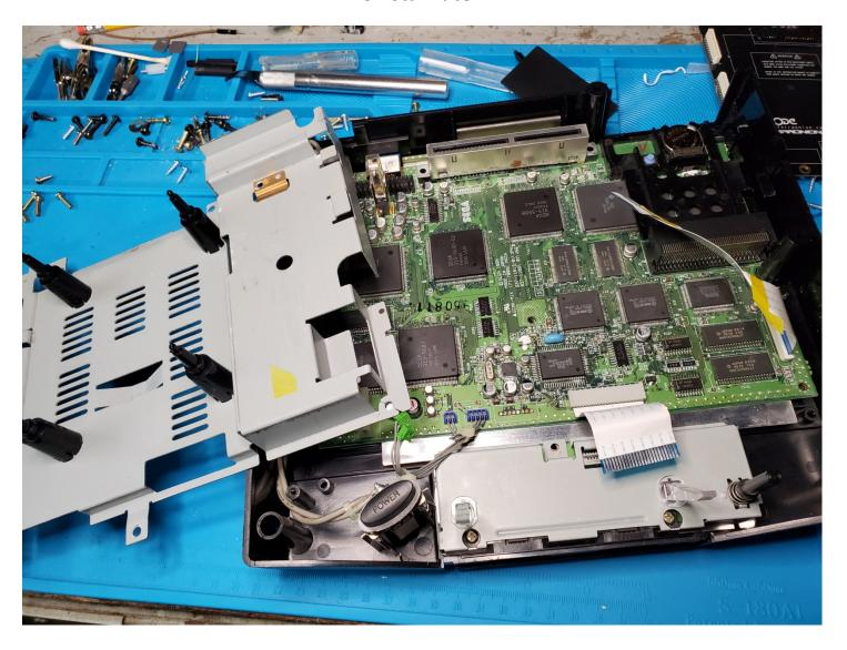
Turn hard metal shielding over and remove 4 screws securing the 4 black ROM mounts. Keep screws.
