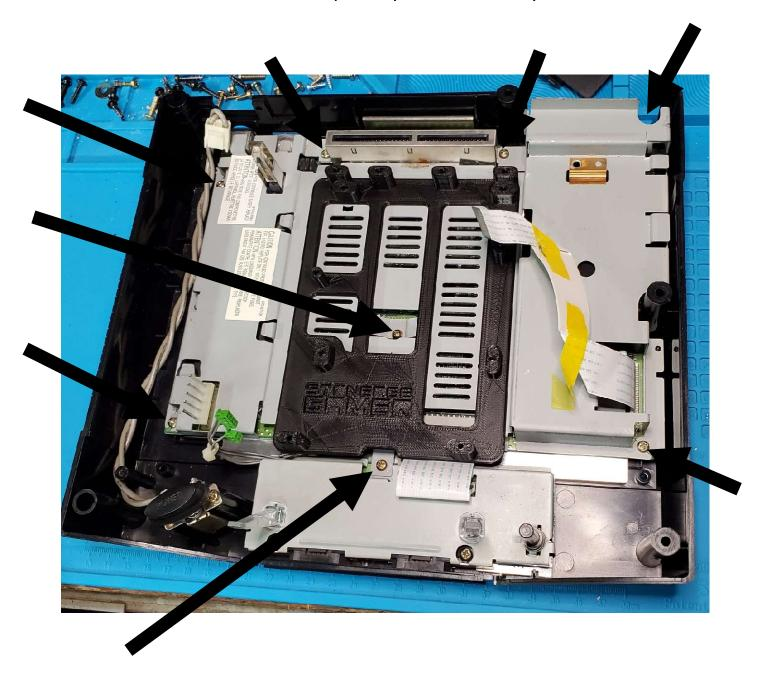
Install MODE using the 4 included screws. Plug in ROM ribbon and ROM connectors to the MODE. Install power supply with 3 screws you removed earlier and power plug from MODE kit.
