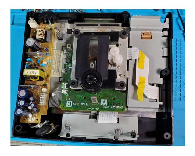
To remove ROM. Disconnect ribbon cables from ROM and screw.
