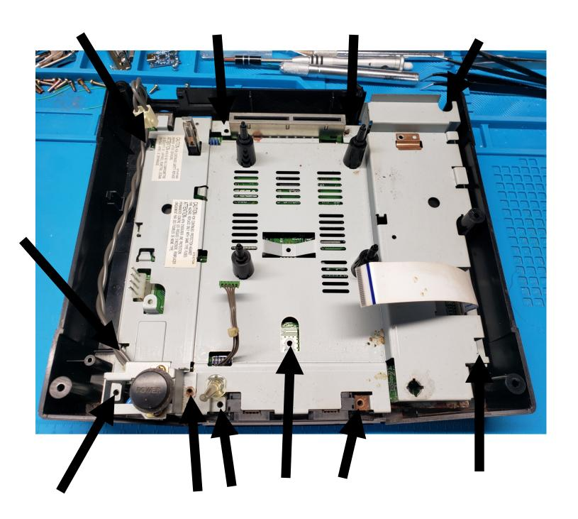
Carefully remove hard metal shielding from Saturn PC board. Remove controller and ROM ribbons if needed. Removal of PC board from case will make it easeier to reinstall later.
