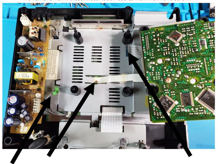
Remove 3 screws from power supply and remove power supply.
