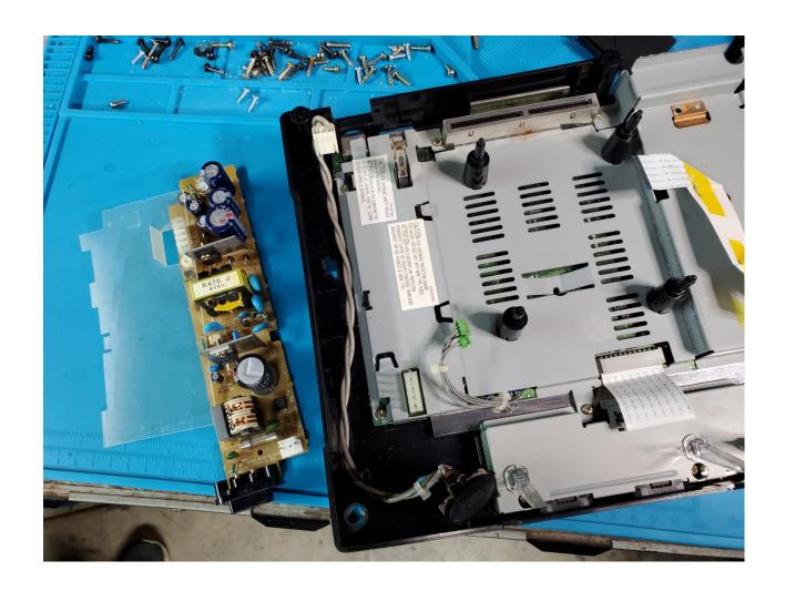
Remove screws securing hard metal shielding and controller port ribbon if you have one. Some Saturns may require removal of power button also.
