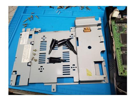
Install SAG MODE mount using the 4 screwes from the 4 ROM mounts.
