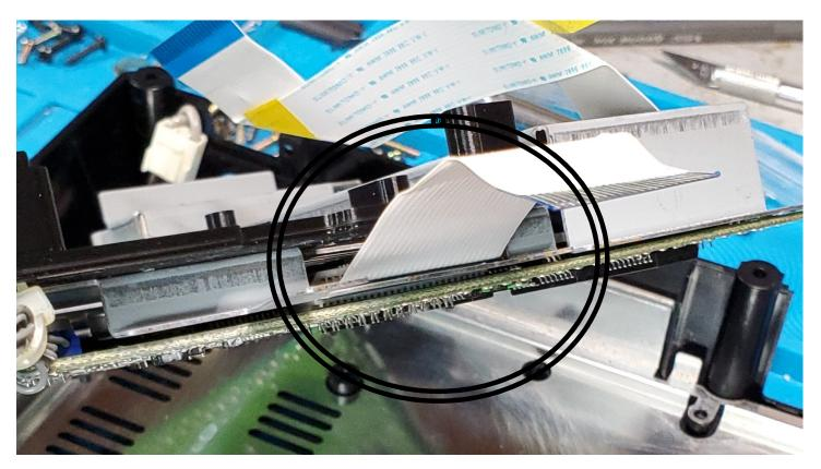
Place Saturn PC board and metal shield into botton of the Saturn case.
