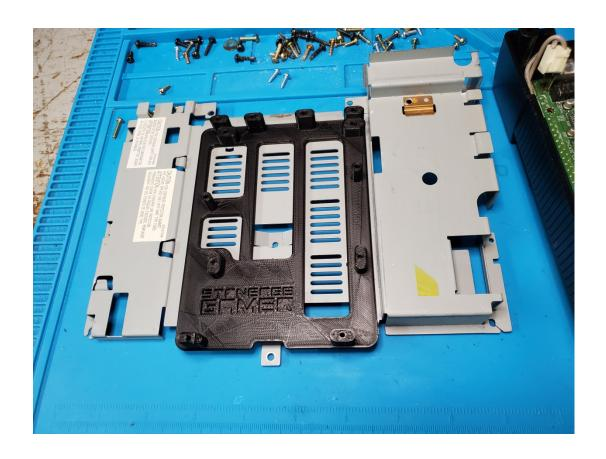
Place assembled hard metal shielding on Saturn PC board. If you have a controller port ribbon now is a good time to install it.
