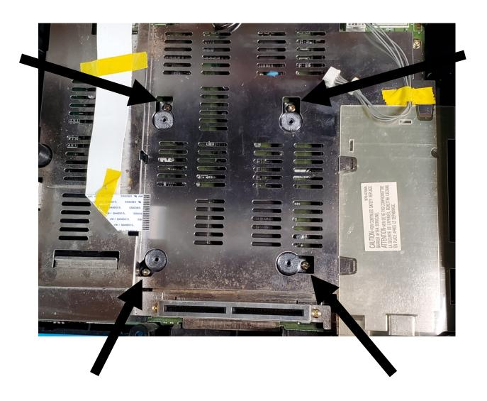
Using 4 of the included screws mount the SAG MODE mount to the standoffs.
