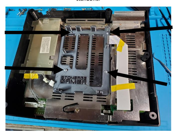
Next using 4 of the included screws mount the MODE to the SAG mount.
