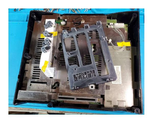
Mount the 4 standoffs to the Saturn using the 4 screws you removed eariler. You may need to remove the flimsy metal shielding.
