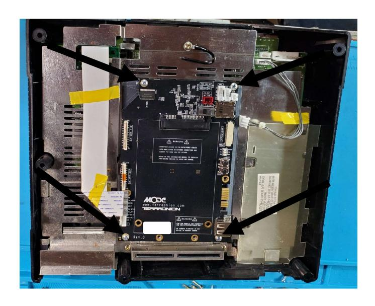
Plug in ribbon and connectors to the mode. Plug in you HDD, Micro SD, or USB. Plug in connectors from top of the case.
