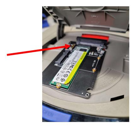
Ensure the switch on M.2 adapter is set to NGFF.
